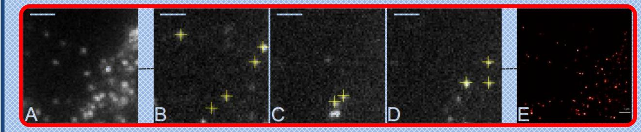
(A) A large number of molecules closely-spaced within the diffraction limit . In order to localise them, dSTORM uses blinking fluorescent dyes. (B-D) Multiple images are recorded ~10,000. In each image a random subset of dye is fluorescing. Localisation of each blink (yellow crosses) is carried out and processed to create (E) a final super-resolution image. Resolution can be resolved to ~20 nm. Scale bars are 2 µm.
