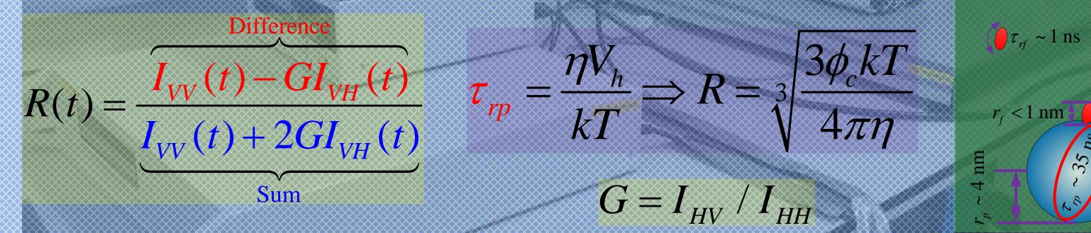
By fitting exponentials to the sum and difference one may find the rotational correlation time, which is the time it takes a nanoparticle to rotate by one radian. From this time, one can calculate the hydrodynamic volume and hence radius.
